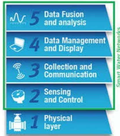
Figure 1. Smart Water Network Architecture
